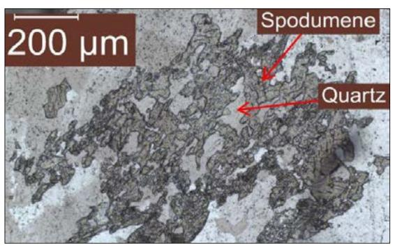
Figure 4-5: Spodumene-quartz intergrowth seen in thin section Source: Scogings et al. (2016)
