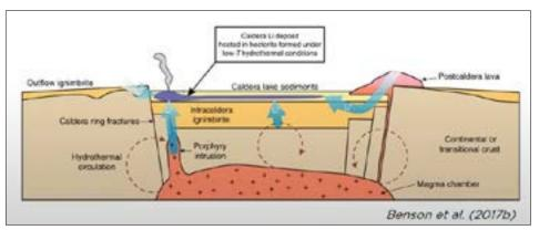
Figure 6-4: Sectional Lithium Model for the McDermitt Caldera (Source: Benson et al.,2017)
