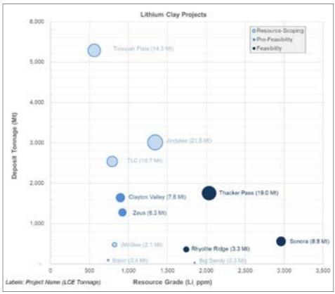
Figure 6-5: Compilation of Lithium Clay Project Tonnages and Grades
