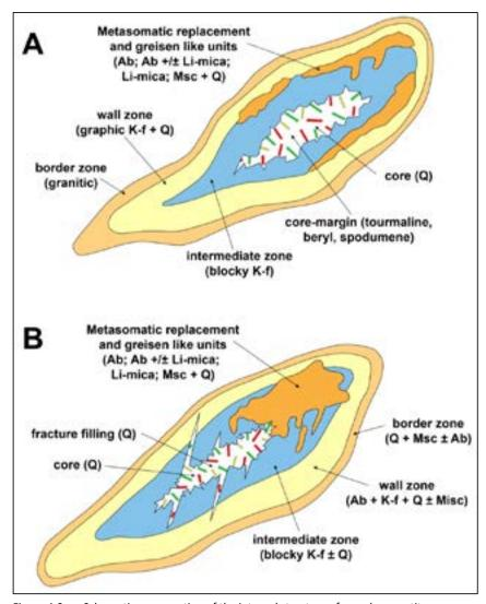
Figure 4-3: Schematic cross-section of the internal structure of zoned pegmatites Source: After Černý (1991)
