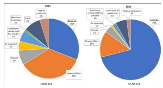
Figure 3-2: Comparison of lithium applications and consumption between 2015 and 2021 Source: USGS, 2016 and 2022
