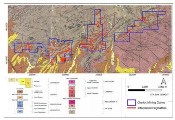
Figure 5-35: Copper Mountain Project - pegmatite targets, interpreted from satellite images Source: Chariot, based on Jacobson (2001) with interpretation of satellite images
