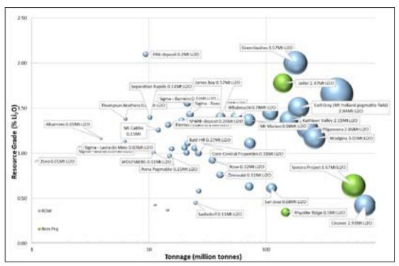
Figure 4-4: Plot of selected global hard-rock lithium deposits (bubble size relative to contained Li<sub>2</sub>O)
